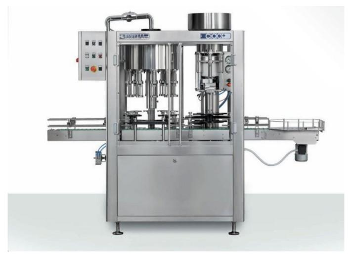
Automatic monoblock for bottling and corking or closing still wine with an aluminum stopper. Filling, corking and closing with an aluminum (monopoly) cap is easy. The device can be equipped with a bottle rinsing station.
