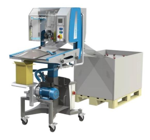
Universal semi-automatic filling machine for bag-in-box bags, which are fed separately (single) or connected together in a belt. Ideal for medium and large productions. The PREMIA WS filler allows you to manage different recipes and maintain high production rates of up to 540 three-liter vacuum bags per hour in "belt" mode.
