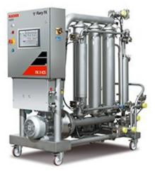
The Flavy X-Wine filter has a reputation in the market for providing the best flow rate for the filtration of the most difficult wines. This result is the result of 30 years of experience in wine filtration. Membrane clogging control combined with a gentle (ultra-low pressure), flexible process and high-efficiency filtration membrane ensures a stable, regular flow rate throughout the entire filtration process.
