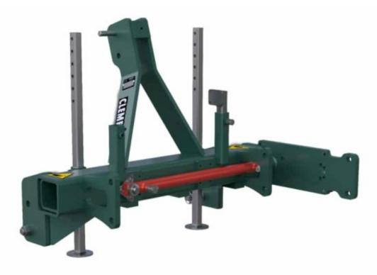
Would you like to work permanently with only a single-sided undervine care device, but as comfortably and safely as possible? For this case we have developed the SB MONO, which can be used for front and rear mounting. The hydraulic width adjustment can be easily converted from right to left. The base frame can be hydraulically adjusted by 500 mm from 960 to 1,460 mm on one side by means of a cylinder, either to the right or to the left.
