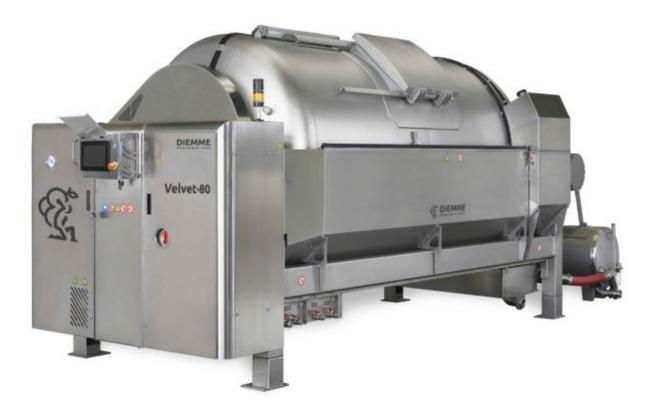
Horizontal pneumatic press with side membrane certified in accordance with current European Directive in force, with closed AISI 304 stainless steel tank. High draining efficiency thanks to mirror-polished channels placed along the internal lateral surface. Simplified
